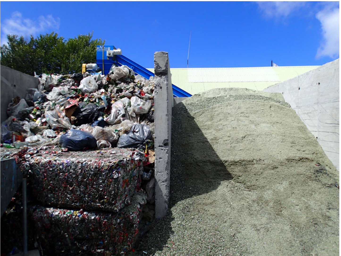
Figure 11. Aluminum cans (left) and ground glass powder (right).
